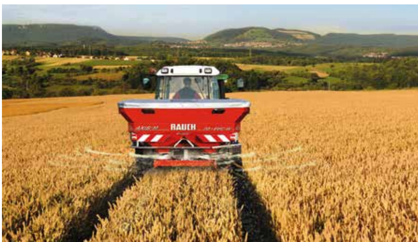
Sowing coated seed with a fertiliser spreader about three weeks before the wheat harvest
