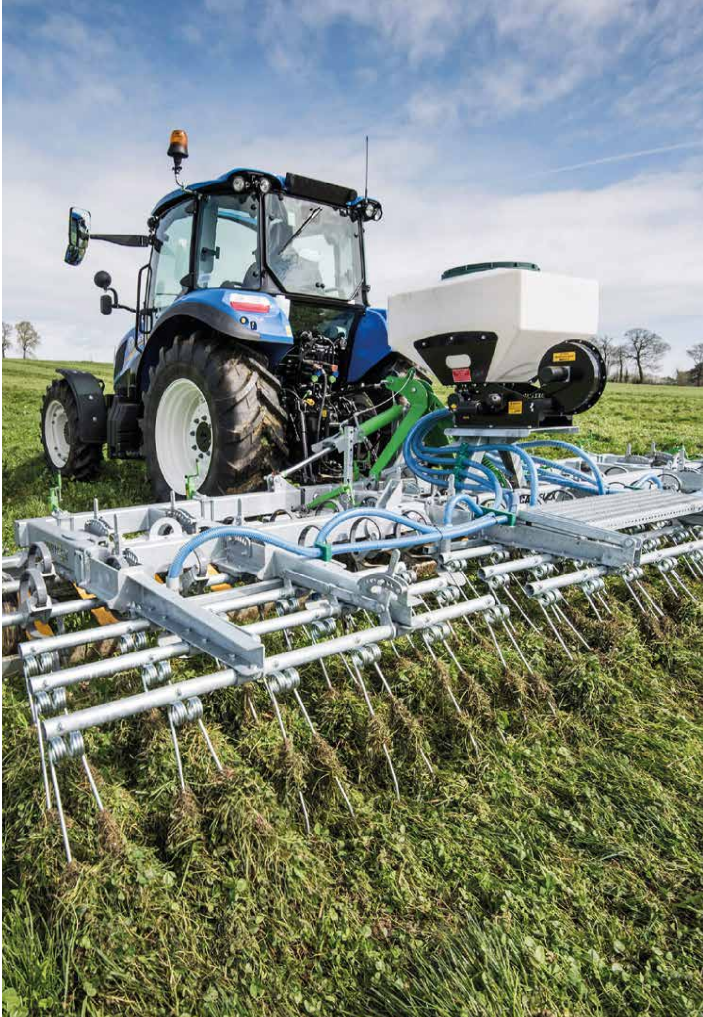
Modern combination equipment helped to combine the advantages of harrows and levellers while carrying out the grassland reseeding.
