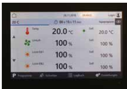
Control unit of an environmental chamber
